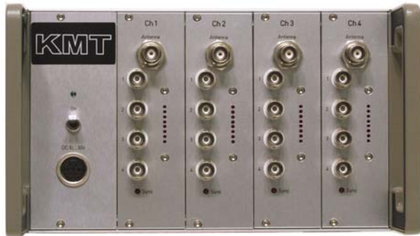
Front view with 4x4 BNC outputs and RF-levels
