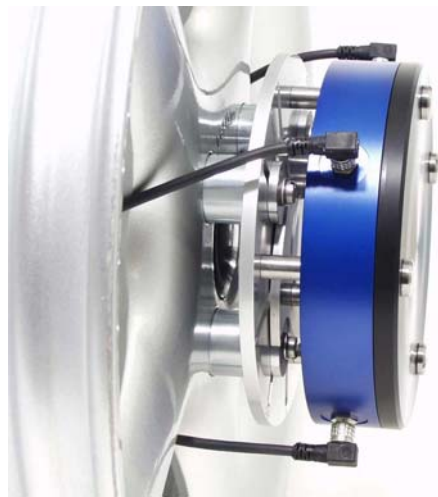
Side view with sensor inputs and mounting plate
