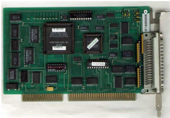
IF16 data acquisition card for ISA slots in desktop computers
